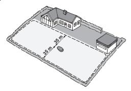
When the Auto Mower's working area borders, e.g. collections of water, driveways and pathways, etc. the boundary wire should be supplemented with a number of posts, edging or a fence with a height of at least 15 cm. This is an additional safety measure to prevent the Auto Mower from running outside of its working area if the boundary wire is installed incorrectly.
