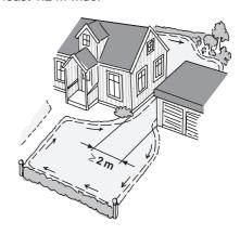
The Auto Mower can mow on slopes with an incline of up to 15°, (rising by 27 cm per metre), but it must be kept away from slopes any steeper than this by the boundary wire.
